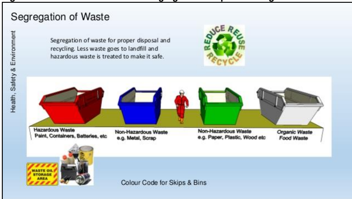
Figure 1 Construction Waste segregation compound design
